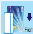
The magnetic strip on the back of the card is swiped vertically through the groove of the card reader from top to bottom.
